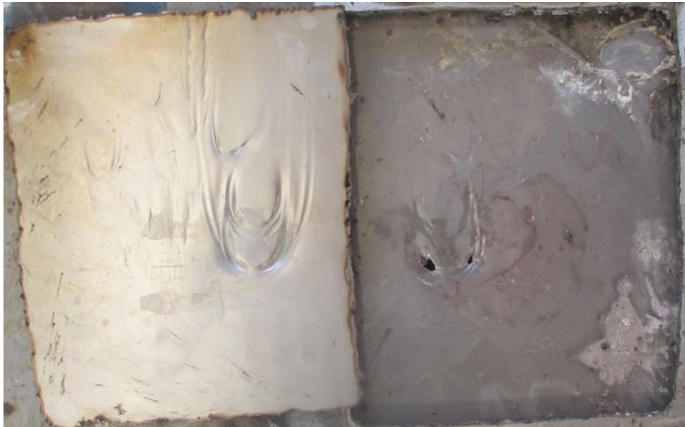
Figure 2. Eroded plate by foreign objects.
